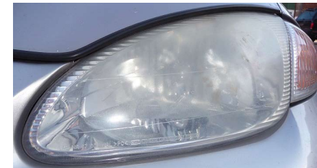
Improper lights: degraded lenses
