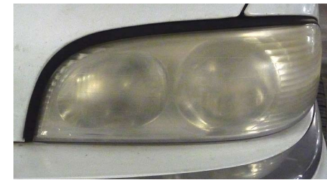
Improper lights: degraded lenses
